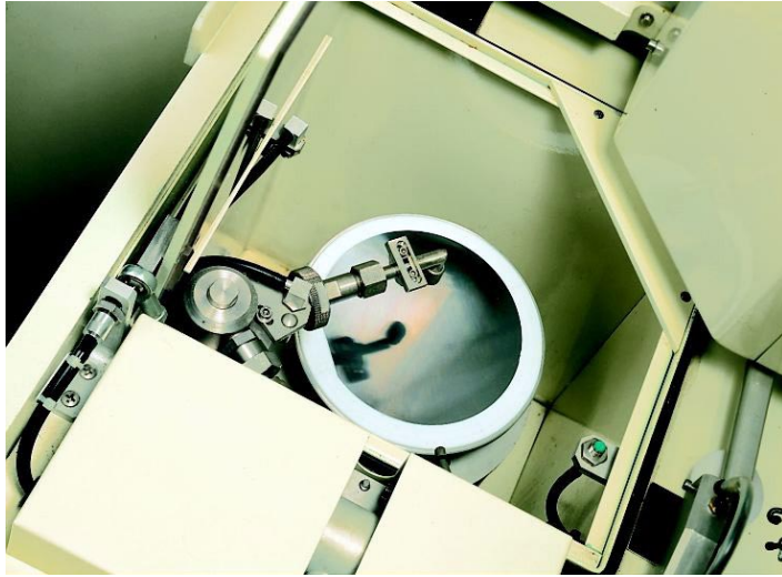
The High-Pressure Cleaning Station Ultraclean Wafers – a Basic Requirement for Subsequent Processing Operations
